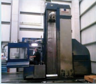
Fresadora SORALUCE FR 14000 cnc HEIDENHAIN TNC 530 . Recorridos 14000x1500x3600 mm. Reconstruida 2012.
