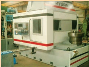
TORNO VERTICAL KRYPTON K023 CNC FAGOR 8035T
