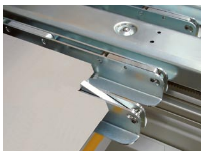
Special gauging system with stop fingers, that can be individually activated
