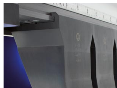
Upper beam tool seat with double slot and key connection
