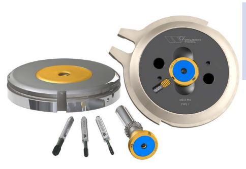
The Wilson Tapping Tool for Trumpf and Pullmax machines can be used to produce a thread in a punched or extruded hole in sheet metal. The Tapping Tool forms the thread rather than cutting, giving a stronger thread and not generating swarf.
