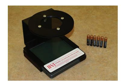
Place the LSA on its side as shown in the picture at right. Remove the battery compartment door, and insert 6 fresh AAA batteries as shown in the picture at right.
