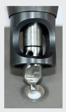
Micro-stop cages used with piloted countersinks helps to ensure a perpendicular approach and enables accurate chamfer depth and diameter.
