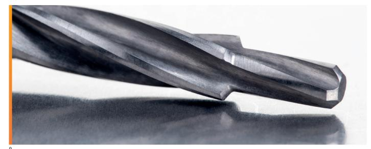
This range of NAS 937 double margin pilot drills is suitable for machining close tolerance holes. Each design has been precision ground with a pilot to maintain concentricity and accuracy. Available in High Speed Steel, Cobalt and Carbide, the drills are available in various shank configurations on request (plain, quick change or 1/4" – 28 threaded shank).
