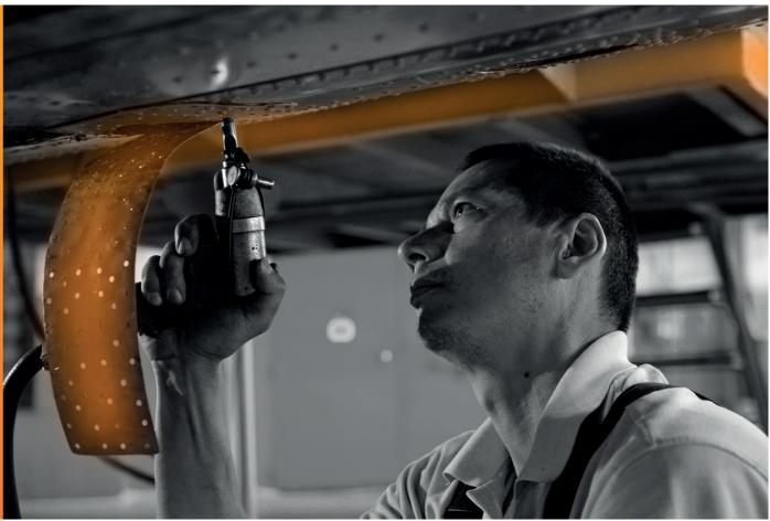
Our assortment of threaded shank drills is available in three varieties, High Speed Steel, Cobalt and Carbide. These are for drilling general to medium duty, low tensile strength materials in confined areas. The Carbide range can be used for drilling composites. A split point geometry, manufactured to NAS specification, reduces thrust forces and improves positional accuracy when hand-drilling.
