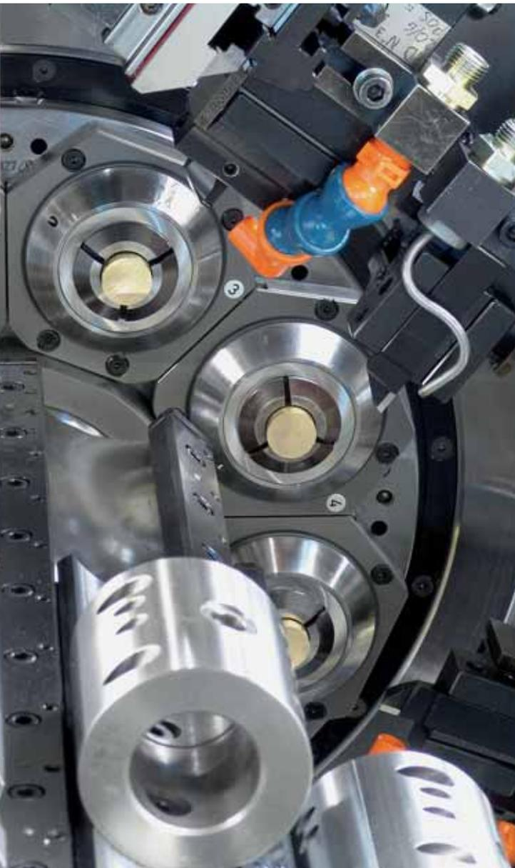
The well proven concept with central sliding block allows the user to mount up to eight independent motor driven frontal spindles. The Y-axis enhances further the possibility for thread milling and grooving from the front side.
