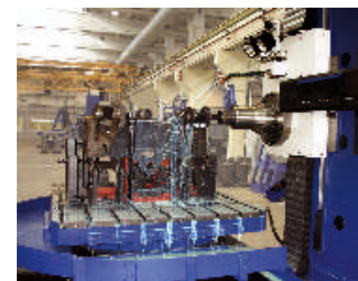
MILLING AND DRILLING OF CRANE PART
