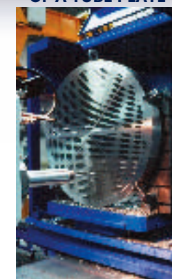
DRILLING OF A TUBE PLATE
