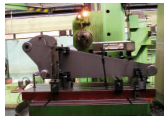
PRODUCTION OF A BUILDING MACHINE ARM
