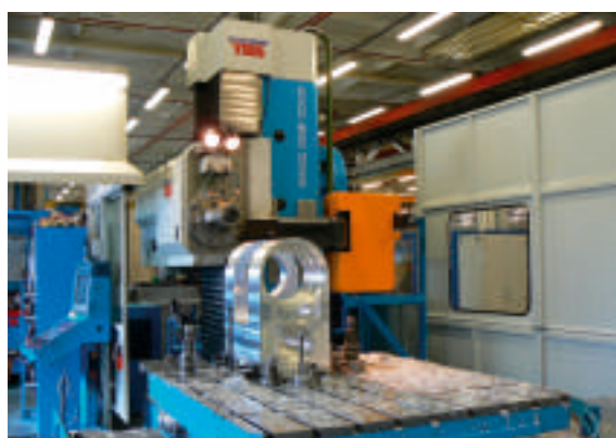
MILLING OF A MILLING HEAD ALUMINIUM BODY
