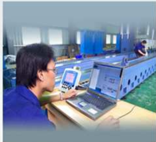
Max. measurement travel 20 m. Straightness is inspected by optical instruments.
