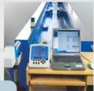
Straightness inspection with collimator
