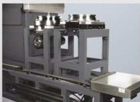
Automatic head magazine (1 head)
