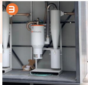
Central filter system with self-cleaning + cyclone.
