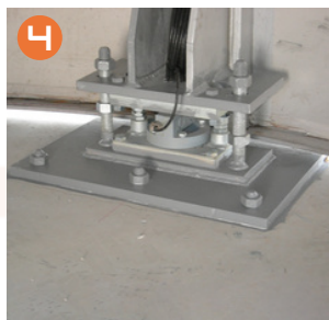
Stock control by weighing (load cells)
