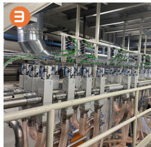
3 Individual material selection valve (VDL).
