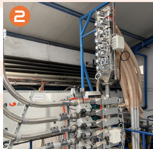
Automatic material selection system (Multiway Valve).
