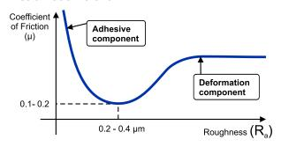
Friction generates a series of local phenomena that have negative effects on elements in relative motion. Metal/polymer, polymer/polymer and polymer/elastomer composites are penalised by adhesion and local micro-deformations favoured by friction-generated heat.
