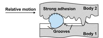
These phenomena lead to the formation of molten polymer and polymer particles (adhesive wear) or debris and grooves (abrasive wear). It is clear that wear is strongly influenced by the degree of finishing of the surfaces involved, i.e., by their roughness. It is not easy to describe a
