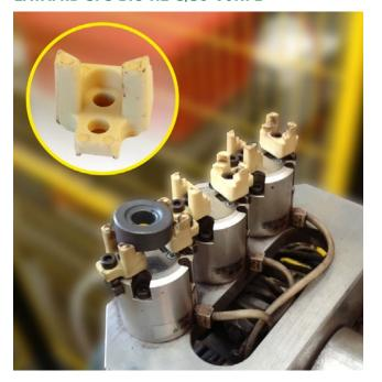
And special grades, e.g. self-lubricating, with aramid fibres:
