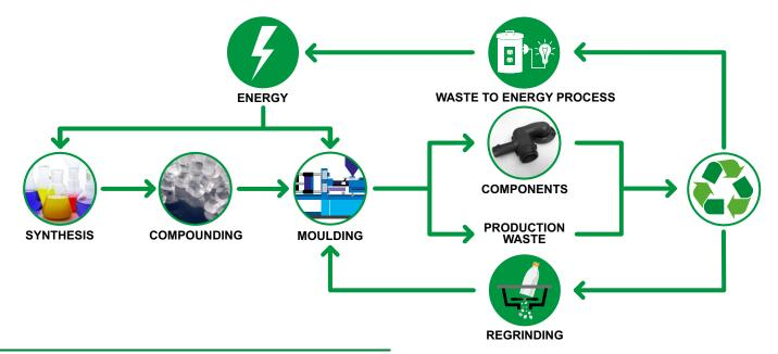
One environmental sustainability avenue that LATI has been pursuing for some time is the use of recycled polymers in its compounds. These are obtained both through traditional mechanical recycling and through chemical recovery, which involves breaking polymers down into monomers and then re-polymerising them.
