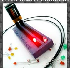
Based on modified **PLA**, thanks to **carbon nanotubes** this material can achieve very low surface resistivity, close to  $10\Omega$ .
