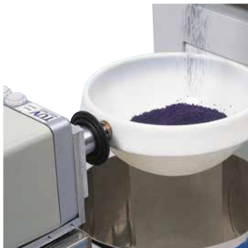
MicroBatch scale: gain-in-weight batching of small ingredient amounts
