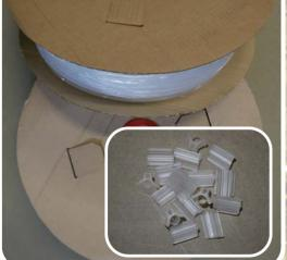
Clips for grafting plants are available in different diameters, and prepares in rollers. The machine automatically supplied with the clip roller, cutting individually the clip at the grafting moment.
