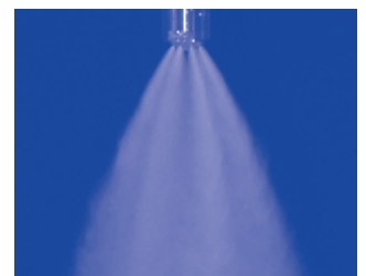
Spray pattern of the VarioJet nozzle
