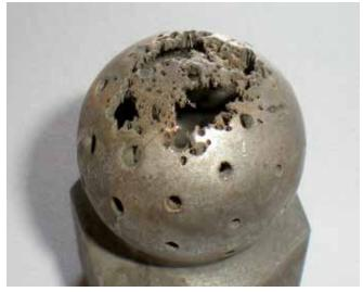
Figure 13: Chemical attack on a spray ball
