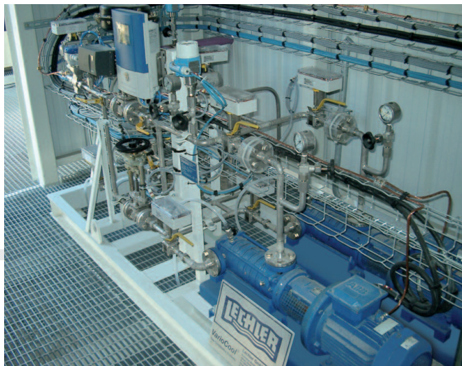
Compact pump and regulating unit for installation in a container
