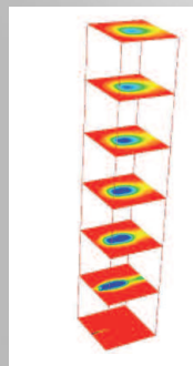
Temperature curve at various levels after the denitrification agent has been injected.
