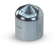
Lechler VarioJet® nozzles atomize according to the principle of internal mixing. With this twin-fluid nozzle, the water is fed in axially via a bore hole.
