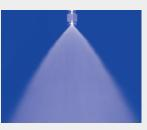
Spray pattern of a single spillback nozzle
