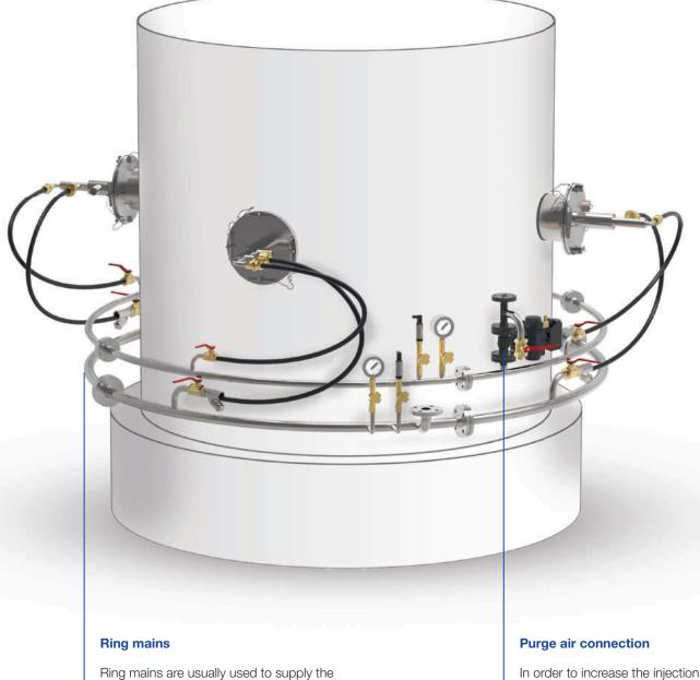
In order to increase the injection turn-down ratio, individual lances or lance groups can be connected or disconnected. If the disconnected lances are in the flue gas duct, the rest of the fluid should be purged. Vaporization and deposits in the lance can be prevented in this way.
