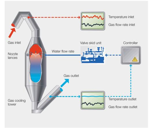
We supply you with completely preassembled and tested valve skid units with defined interfaces. Each of the components is perfectly tailored to the function of the nozzle lances and their on-site connections.
