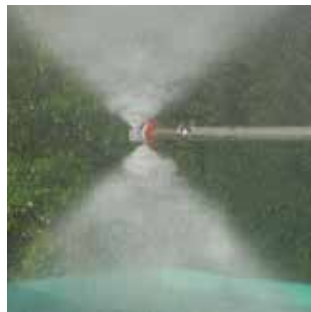
Spray pattern with two counter rotating full cones
