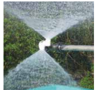
Spray pattern with two counter rotating hollow cones
