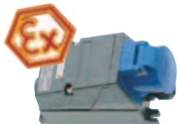
Explosion-proof socket, 3-pole CEE-type socket, explosion-proof to II 2 G EEx de IIC T6, 220-240 Volt, protected to IP 65
