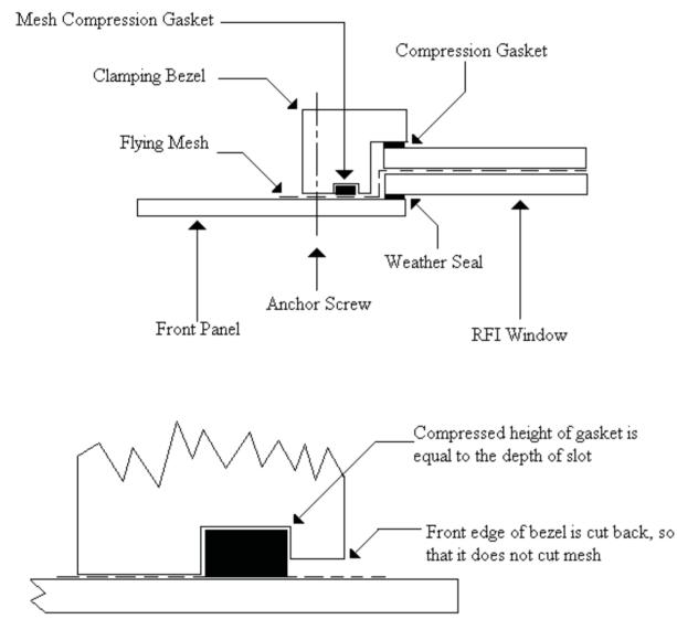
The rear surface of the front panel must be free of paint and should have a conductive plating applied for mesh contact
