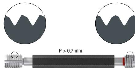
The gauging of the saw-tooth profile works on the same principle, with the only difference that both the go and the no-go plug gauge have to be used in the correct direction.
