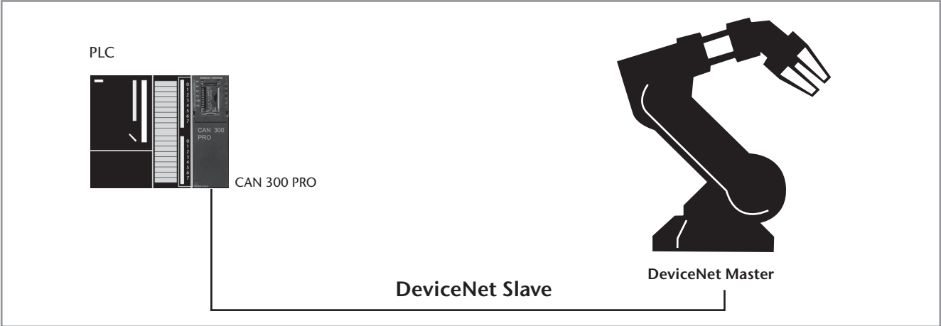
Application Example CAN 300 PRO as a DeviceNet Slave
