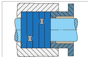
One or more rings have been cut too short causing the following ring to be pressed into the empty space.
