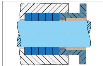
Shaft and bore axis are offset, and this imbalance causes severe wear and scoring.
