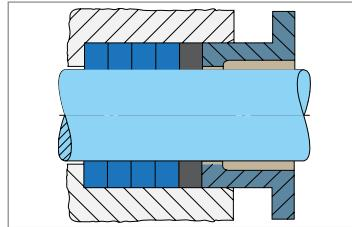
Bad end ring installation. The gland pressure required for the sealing is unable to be distributed evenly through the packing set (insufficient gland pressure).
