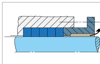
The play between shaft and gland follower is too large. Installing the correct anti-extrusion rings should solve the problem.
