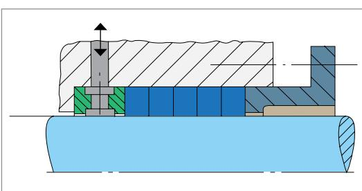
Flushing for the protection of packing arrangements.
