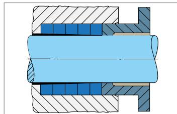
The shaft bearings are faulty, causing the shaft to run out of true and damage the packing.
