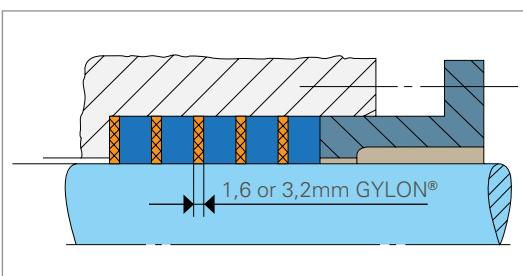
The GYLON® discs between the individual packing rings stop the extrusion of packing and lubricant.
