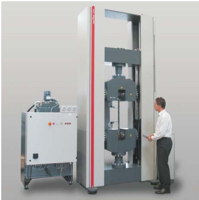
Figure: Zwick Z1200Y with hydraulic grips
