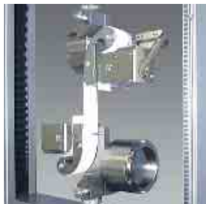
Pneumatic action capstan grips
