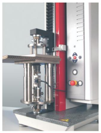
Fig. 2: LPET-Test in a testing machine
