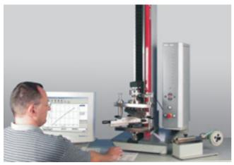
Fig. 1: Internal Bond Test - test rig and sample preparation unit (bottom right)
