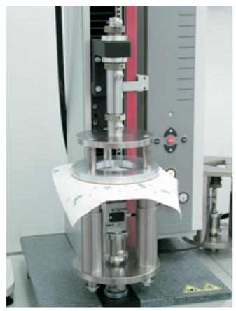
Fig. 1: Burst test on tissue
