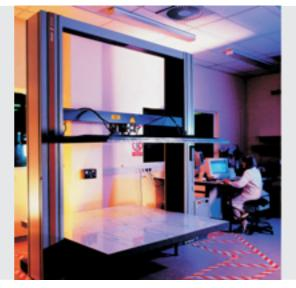
Fig. 2: Box-crush tester for specimen up to a footprint of 2 m by 2 m (authorized by SCA Packaging Research, European Technical Centre, Aylesford)
