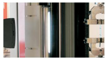
Fig. 3: videoXtens measures extension and transverse strain
