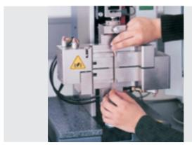
Fig. 1: Strip crush test grips
