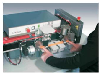
Fig 1: zwicki, equipped with horizontal test space and automatic test start
