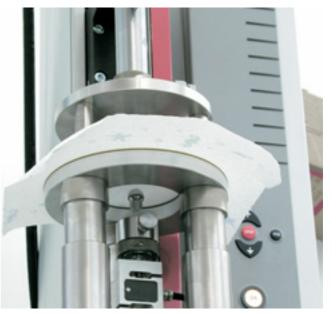
Fig. 3: Puncture test rig configuration
