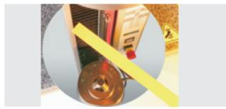
Fig. 2: Compressibility test using zwicki
