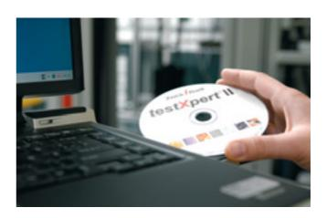
You can record the test procedure with a video camera or an USB webcam. *testXpert*® II saves the recorded images **synchronized with the measuring data**. The visual recording shows, for example, when, how and where the specimen necks, buckles or changes color.
