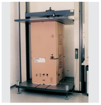
Fig. 2: Measurement of the buckling of a filled, folded box
