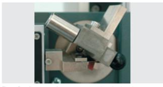
Fig. 1: Bending test on fine paper at 1 mm bending length
