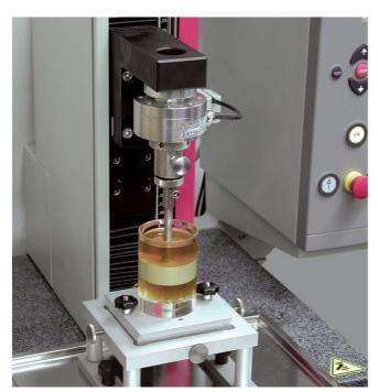
Fig. 1: Zwick Roell back extrusion rig
