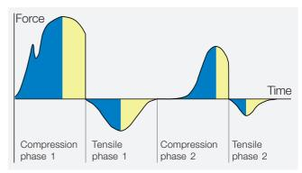
Fig. 1: Principle sequence of a cyclic test (2x mastication) / procedure of instrumental texture profile analysis (TPA)
