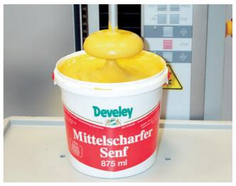
Fig. 2: Viscosity measurement directly in the container
