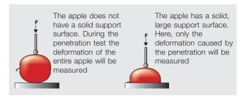
Fig. 3: Application of force to the specimen
