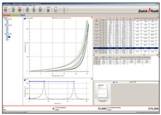
Fig 1: testXpert® II provides a quick and good overview over all test results. During the test you can watch the curve online on the display
