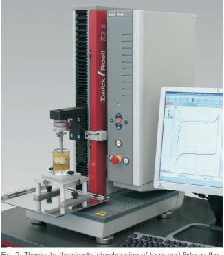
Fig. 2: Thanks to the simple interchanging of tools and fixtures the ProLine Z0.5 can also be used for viscosity tests
