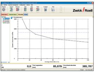
Fig. 1: Only one test is required to determine and represent the viscosities over the entire shear rate
