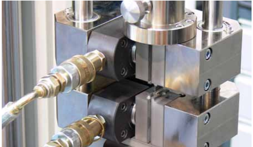
Fig. 3: The HCCF - Hydraulic Composites Compression Fixture - is used for shear loading and combined loading
