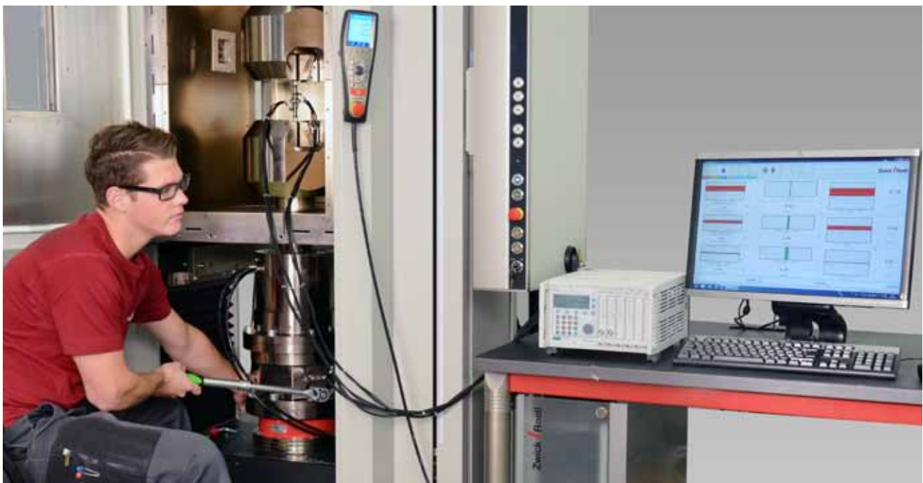
Fig. 1: Testing machine alignment and verification by a Zwick technician using an alignment equipment in accordance with ASTM E 1012.
