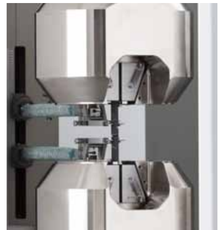
Fig. 1: Centrally closing wedge grips, laterally adjustable wedge-screw grips and hydraulic wedge grips with a wide range of jaws are available for testing all kinds of laminates.
