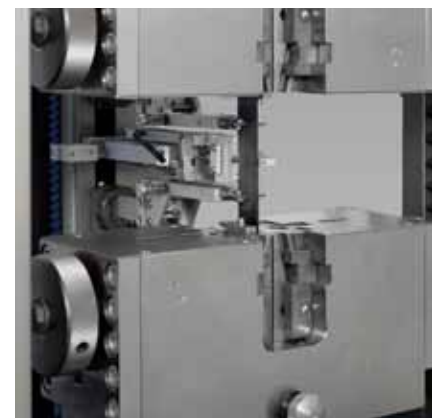
Fig. 5: Measuring shear deformation in two planes using makroXtens
