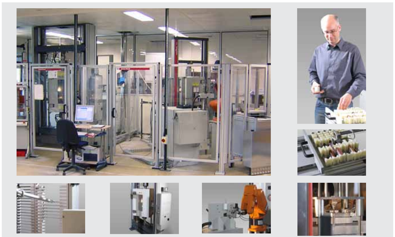
Fig. 1: Fully automatic testing system with two load frames for tensile, OHT, FHT, IPS, lap-shear tests, ILSS, load bearing and flexure tests over a wide temperature range
