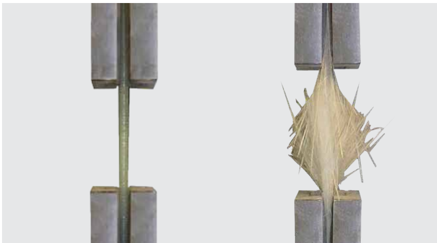
Fig. 1: Valid fiber failures in the free length between grips achieved by soft load application.
