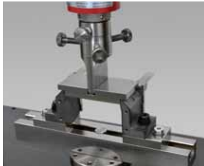
Fig. 3: Loading nose and supports are aligned under load
