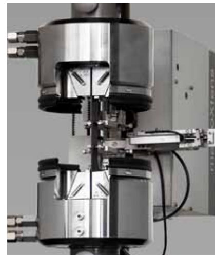
Fig. 5: In-plane shear (IPS) at ambient: makroXtens with reduction-in-width monitor
