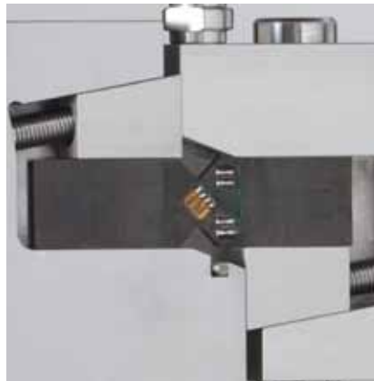
Fig. 2: Strain gages applied directly to the specimen
