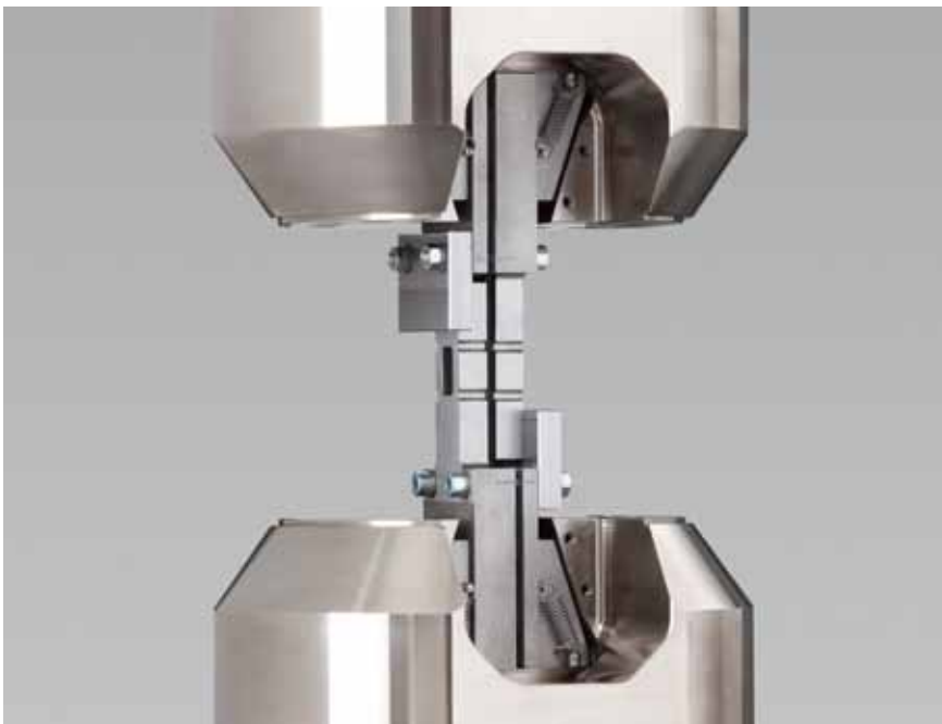
Fig. 1: Pin-bearing strength, single-shear, in compression test, Method B to ASTM D 5961
