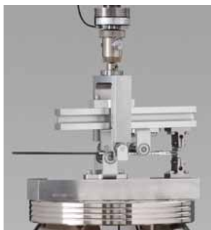
Fig. 3: Adjustable Mode I / Mode II proportions in mixed mode bending (MMB) method
