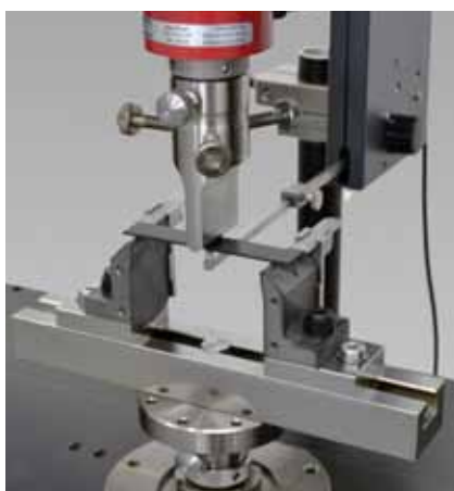
Fig. 1: Mode II energy release rate G_{IIc} , end notch flexure (ENF) method
