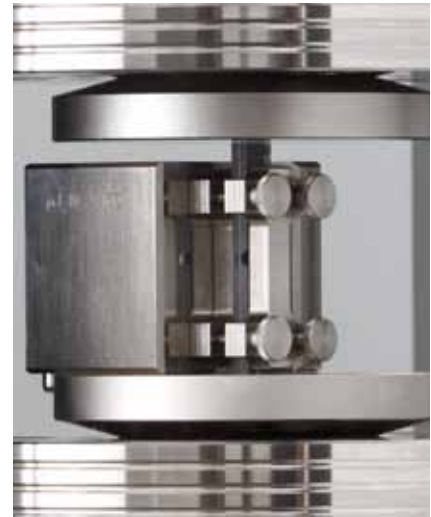
Fig. 2: End-loading compression test fixture to EN 2850 and ASTM D 695 (modified Boeing). The support block is centered to the compression axis by end stops.
