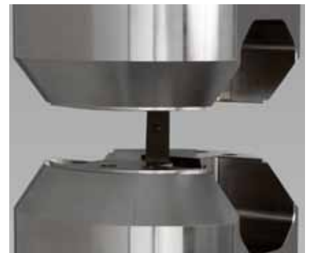
Fig. 2: Tensile tests are performed as plain tensile in fiber direction (0°), perpendicular (90°), and on multi-directional laminates also as open-hole tensile (OHT) or filled-hole tensile (FHT) tests.
