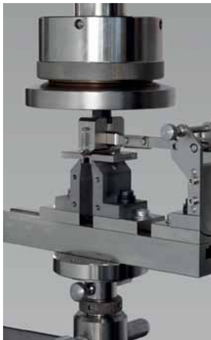
Fig. 3: Setting gage with variable support span
