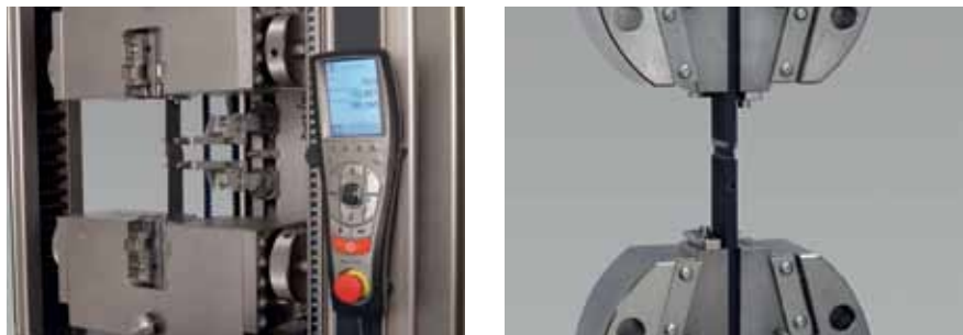
Fig. 2: Specimen grips must have lateral adjustment capability for testing simple single-lap shear specimens (left). Right: slotted double lap-shear specimen.
