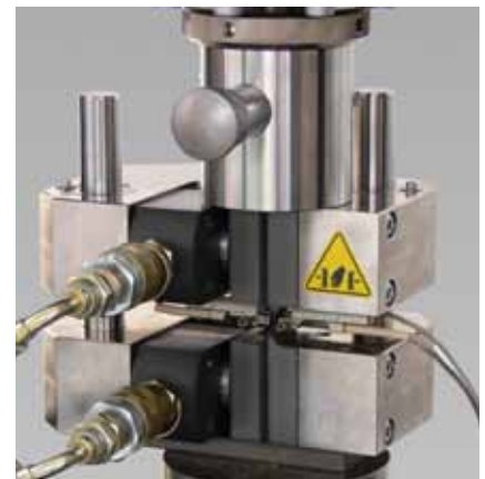
Fig. 6: Various standards permit strain measurement using clip-on extensometers
