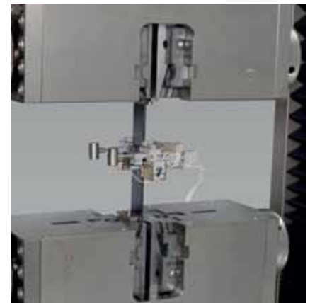
Fig. 4: Measuring shear deformation with a biaxial clip-on extensometer
