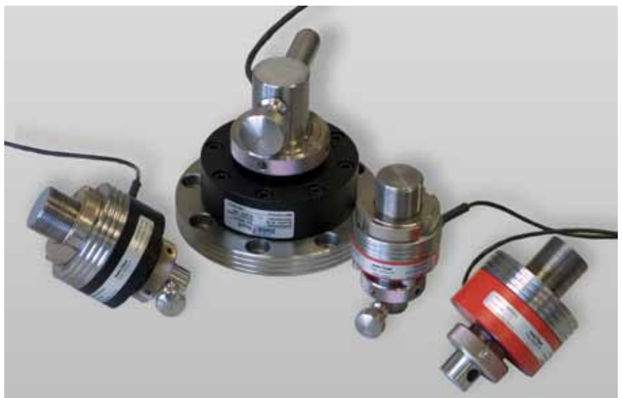
Fig. 1: Load cells for the most exacting quality requirements at Zwick: left, a load cell from the Xforce range employing multiple beams; centre, Xforce HP model using the ring-torsion measurement principle
