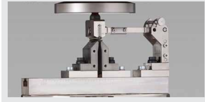
Fig. 2: ILSS fixture. The side-mounted upper-anvil guide-arm ensures exact central force application
