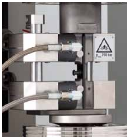
Fig. 2: The HCCF is also suitable for open-hole compression tests to Airbus standards
