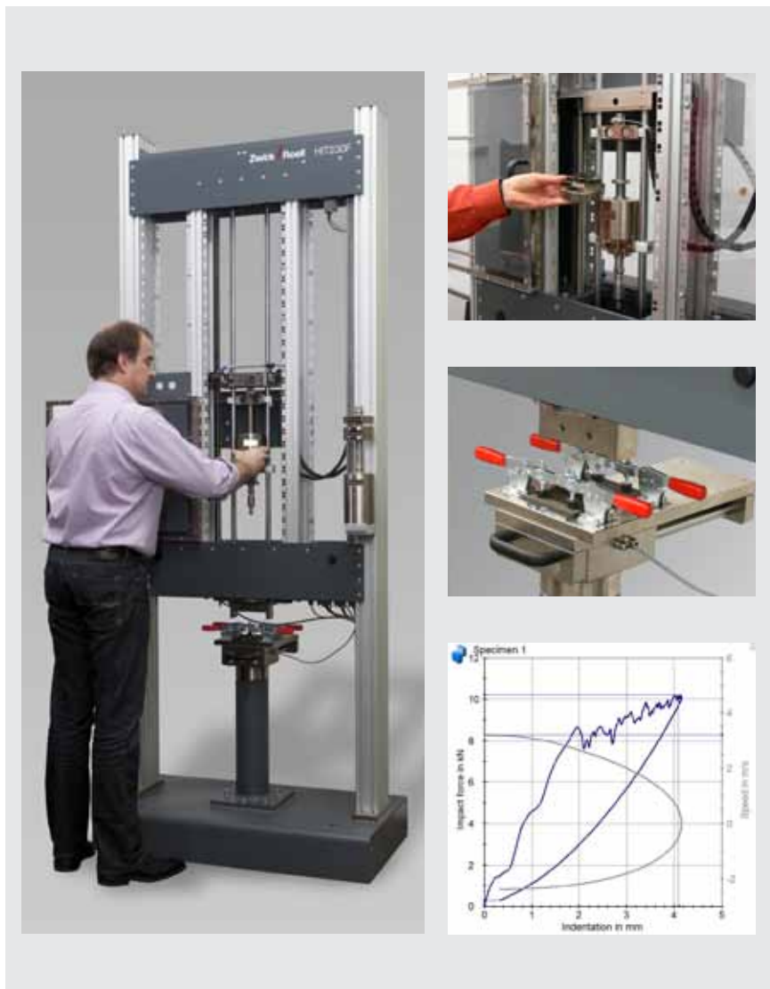
Fig. 1: The instrumented HIT 230F drop-weight tester is used for pre-damaging test panels for the CAI test. The force-travel diagram shows the damage progression.
