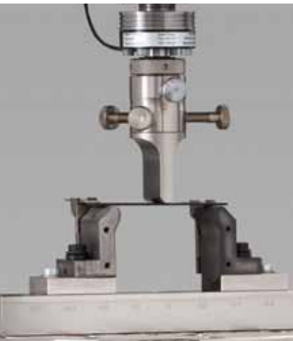
Fig. 2: Three-point flexure test with indirect deflection measurement via crosshead travel
