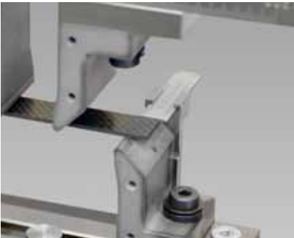
Fig. 1: Exact positioning of specimen via end-stops
