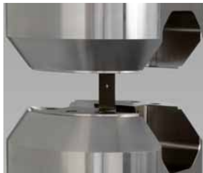
Fig. 2: Tensile tests are performed as plain tensile in fiber direction (0°), perpendicular (90°), and on multi-directional laminates also as open-hole tensile (OHT) or filled-hole tensile (FHT) tests.
