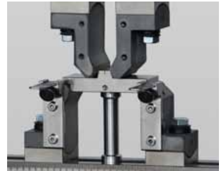
Fig. 5: A special jig is used in the four-point flexure arrangement
