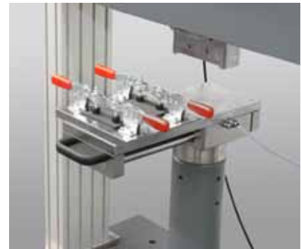
Fig. 3: The CAI specimen is securely held in the drop-weight tester
