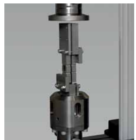
Fig. 5: OHC and FHC compression tests to ASTM require an anti-buckling guide, used both in shear loading with hydraulic grips and in end loading between compression platens
