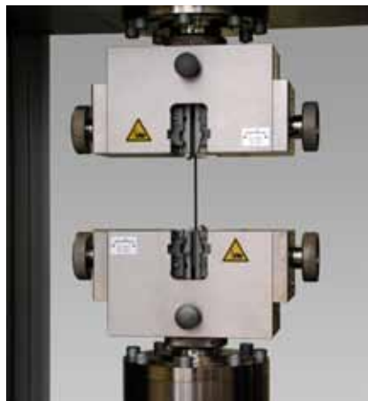
Fig. 1: Centrally closing wedge grips, laterally adjustable wedge-screw grips and hydraulic wedge grips with a wide range of jaws are available for testing all kinds of laminates.
