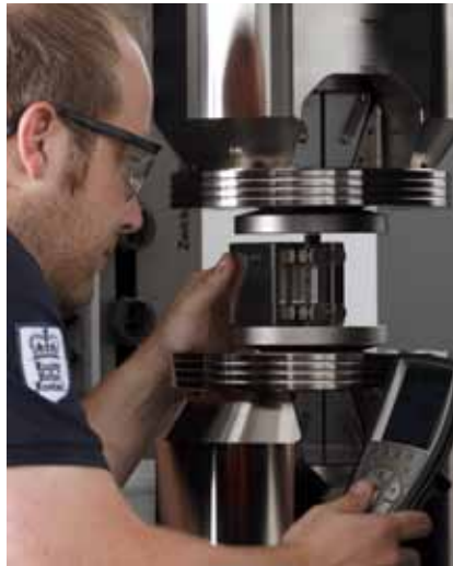
Fig. 2: End-loading compression test fixture to EN 2850 and ASTM D 695 (modified Boeing). The support block is centered to the compression axis by end stops.
