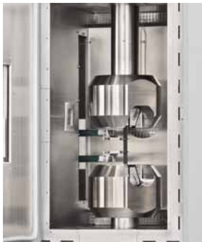
Fig. 2: Tensile tests in temperature chamber, makroXtens with long feeler arms
