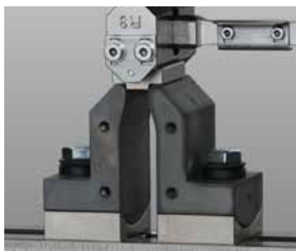
Fig. 1: Standard 10 mm setting gage for exact alignment
