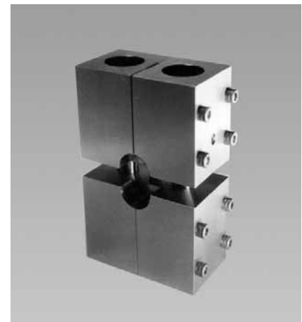
Fig. 4: Combined loading compression test fixture to ASTM D 6641 (© Wyoming Test Fixture Inc.)
