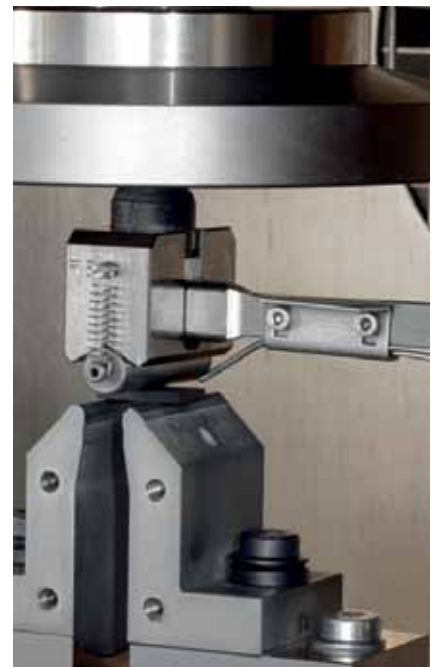
Fig. 4: Mounting a temperature sensor close to the specimen
