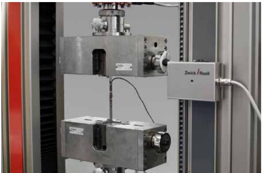
Fig. 4: Direct connection of strain gages to testControl II via a ready-configured control box
