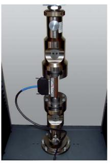
Fig. 1: Configuration for alignment verification
