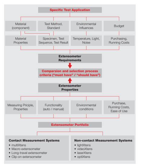
Fig. 4: Selection process of extensometers
