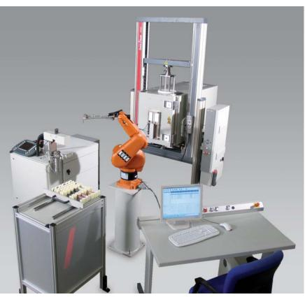
Fig.2: Robotic testing system for automatic flexure tests on composites
