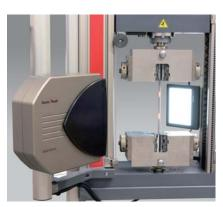
Fig. 3: laserXtens with round specimen
