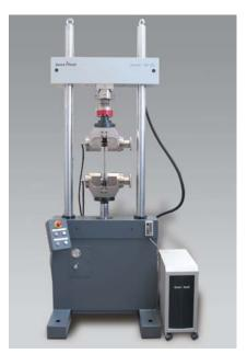
Fig. 4: Servo-hydraulic testing machine Amsler HA
