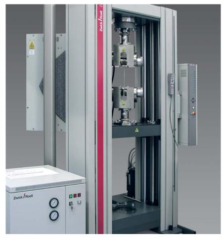
Fig. 1: Materials testing machine Allround-Line Z250
