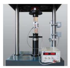
Fig. 3: CT specimen in Vibrophore (HFP)
