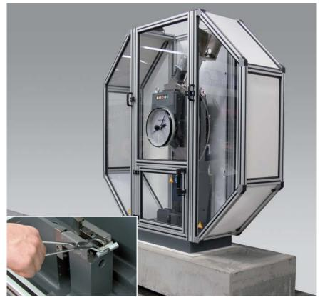
Fig. 2: RKP 450 pendulum impact tester (Inset: anvil)
