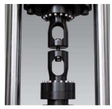
Fig. 2: Fatigue test on bolts/screws
