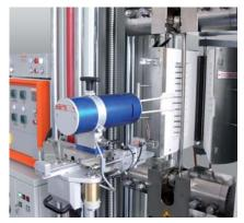
Fig. 1: High-temperature tensile test up to  $1600^{\circ}$  C
