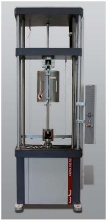
Fig. 3: Creep testing machine
