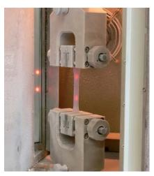
Fig. 4: Tensile test in temperature chamber up to -70  $^{\circ}\mathrm{C}$
