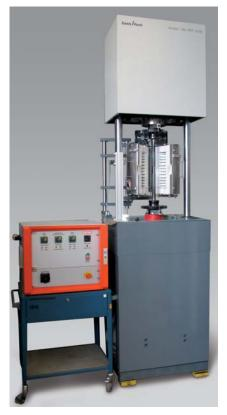
Fig. 1: Vibrophore with high-temperature furnace
