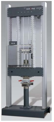
Fig. 1: Drop-weight tester HIT230F
