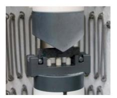
Fig. 2: High-temperature flexure test in furnace
