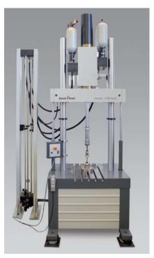
Fig. 3: High-speed testing machine Amsler HTM
