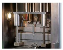
Fig. 4: Flexure test device
