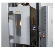
Fig. 1: Temeperature chamber for composite tensile tests
