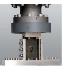
Fig. 2: Compression after impact test device
