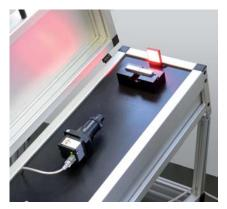
Fig. 1: Optical measurement system notch vision
