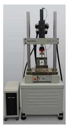
Fig. 1: Servo-hydraulic testing machine Amsler HC10
