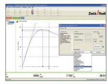
Fig 5: testXpert® II with faded in virtual testing machine
