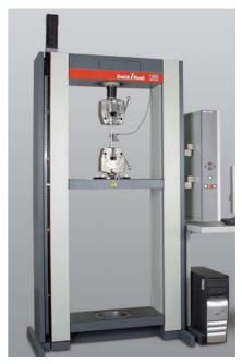
Fig 2: Materials testing machine Zwick 1455 after the modernization with *testControl*
