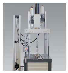
Fig 4: High-speed testing machine HTM
