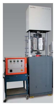
Fig 1: Fatigue strength testing under high temperature
