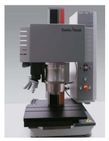
Fig 4: Hardness testing machine Zwick ZHU2.5/Z2.5
