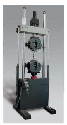
Fig 1: Fatigue testing machine Amsler HB 250
