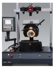
Fig 2: Sheet metal testing machine Fmax 1000 kN with camera to determine the FLC (forming limit curve)
