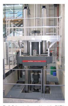
Fig 2: Fatigue testing machine at the RWTH Aachen, Germany (Fmax 5000 kN, static, Fmax 4000 kN dynamic)
