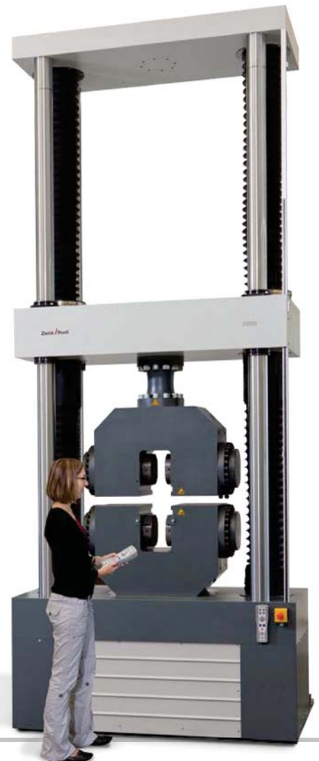
For major challenges. High-capacity machines up to 2,500 kN
