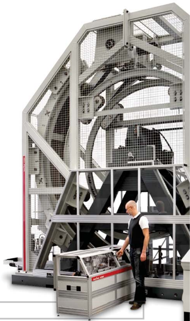
The world's biggest pendulum impact tester, used for impact tensile tests on pipeline materials
