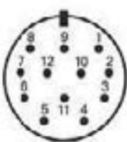
Male connector on the incremental encoder side
