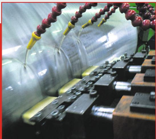
Electrical superfinishing attachment for mounting on large carrier machines for superfinishing of ground and turned surfaces. Well suited for superfinishing of large rollers to a mirror finish and for the simultaneous processing of several tracks.
