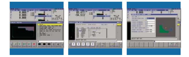
Manual Guide i is the very latest in conversational programming from FANUC and it allows the operator to generate part programs quickly and efficiently through the use of easy to understand conversational cycle prompts.
