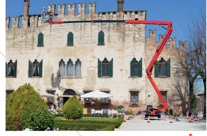
Length of the machine in transport configuration is less than 6m thanks to the detachable basket.
