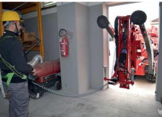
Height of the machine in transport configuration is less than 2m allowing easy passage through the doors.
