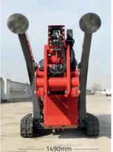
Incredible widening of the undercarriage, from 990mm allowing easy passage through narrow and cramped places, to 1490mm for an enhanced lateral stability.
