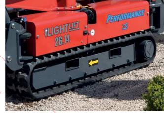
Large forklift pockets to allow easy lifting with forklift or tele-handler to load, unload and transport the machine.
