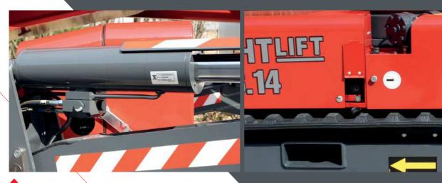
Outrigger block valves doubled for safety, also protected from accidental impact. Auxiliary connector for external devices, telematics and fleet tracking.
