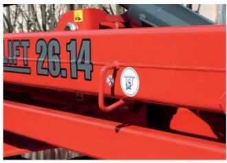
Heavy Duty anchor hooks for improved safety in transport.
