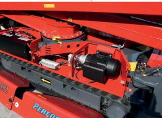
110V-220V electric motor with improved torque.
