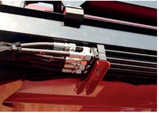
New Zistaplex® hydraulic hose treatment, anticorrosive up to 600 hours in salt spray tests.
