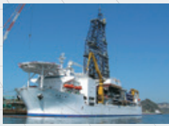
2005 • Constructed deep sea drilling vessel "CHIKYU," which has the capacity to drill 7,000m under the seabed
