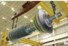
2011 • A "J-Series" gas turbine, with the world's highest efficiency, achieved the world's highest turbine inlet temperature of 1,600 degrees Celsius (°C) during the verification test.
