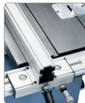
The integrated loupe at the rip fence afford an exact read-off of the adjusted cutting width, HBS 500 N additional with fine adjustment.
