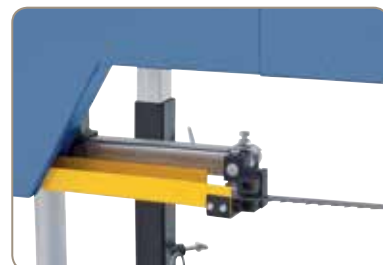
Precise guided bandsaw blade and coolant supply for optimal cutting results
