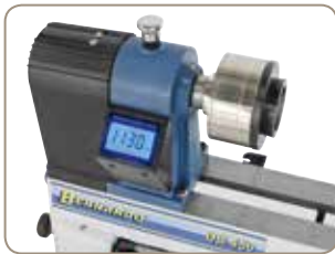
LED display allows for convenient speed readout.
