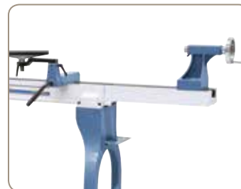
The optionally available outboard turning device (Ø 720 mm) can also be used as bed extension (1200 mm)
