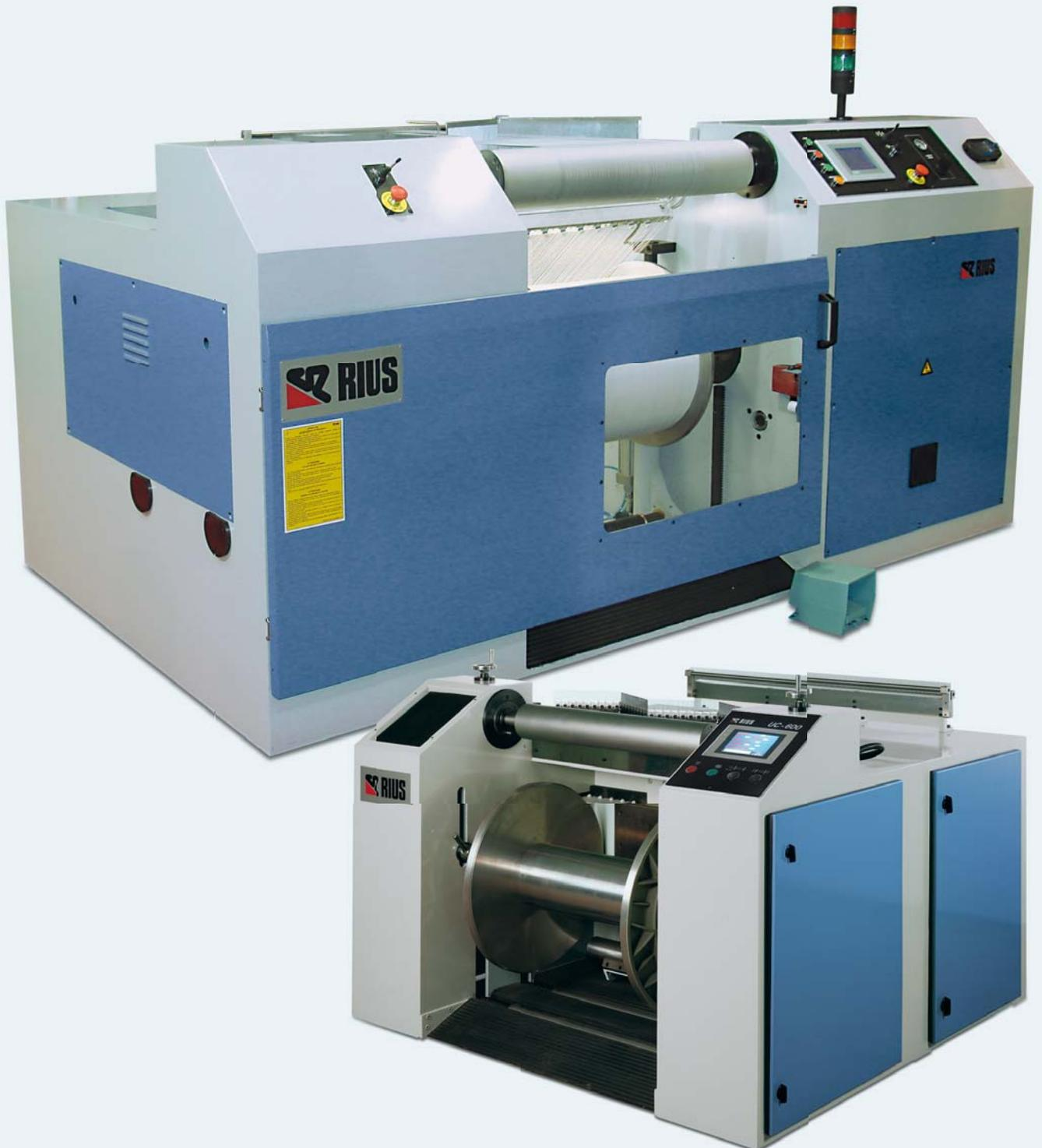
Warping machine driven by PLC and computer touch screen.
