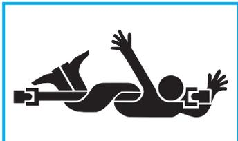
Keep clear of the work area and rotating parts. Do not wear loose clothing, jewelry, or hair that could become entangled with the driveline. Contact with rotating parts can cause serious injury or death.
