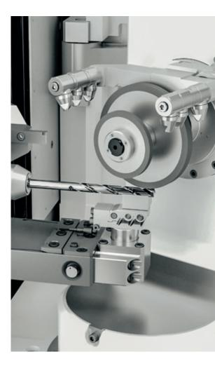
////// STEADY REST WITH AUTOMATIC STROKE ensures an optimal grinding result for longer tools
