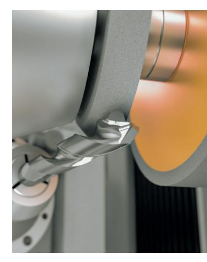
////// MACHINING CARBIDE DRILLS
