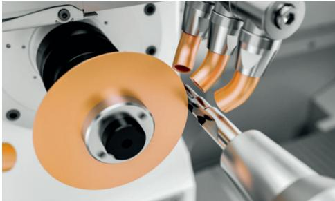
////// MACHINING A PCD STEP DRILL
