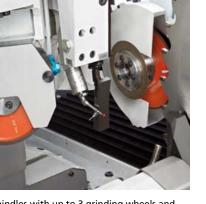
Grinding of chip breaker groove.
