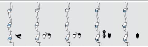
All common tooth geometries for wood and metal cutting are integrated in the standard machine.
