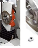
Grinding of chip breaker groove.
