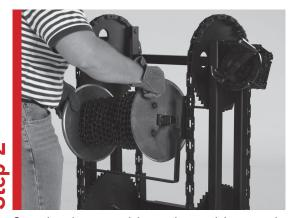
Set clutch assembly and spool into rack.
