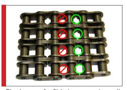
Check gauge for fit between any two roller links. (Perform with chain in tension.)
