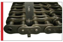
If the gauge step fits through the checkpoint, the chain is worn out and needs to be replaced.
