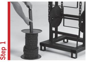
Insert square clutched shaft in roller chain spool.
