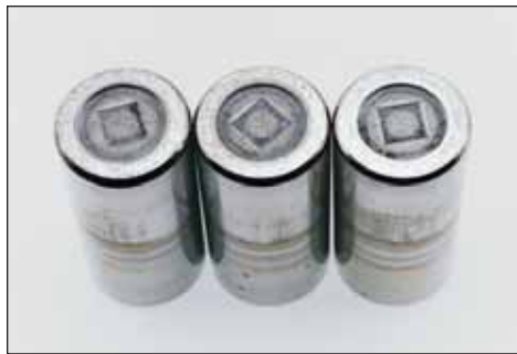
Roller end scoring – Metal-to-metal contact from breakdown of lubricant film.
