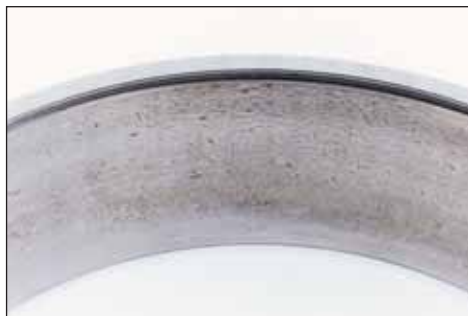
Bruising – Debris from other fatigued parts, inadequate sealing, or poor maintenance.
