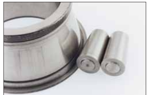
Abrasive wear – Fine abrasive particle contamination.
