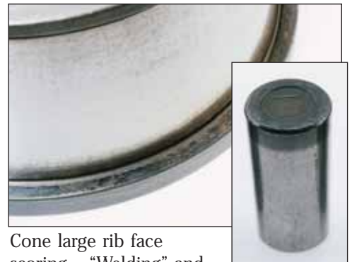
Roller end scoring – Metal-to-metal contact from breakdown of lubricant film.
