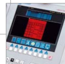
Punching head rotation Index equipment and also stripper height adjustment
