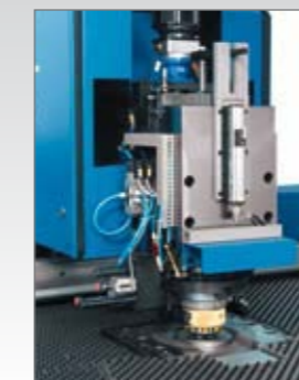
Punching head rotation Solid construction with DC motor and measuring system
