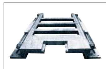
Robust construction Widely spaced ball screw and linear guides guarantee positioning accuracy and repeatability.
