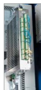
Industrial CPU with RS232 and Modem connection. As an option also available with expanded memory and USB or wireless LAN.
