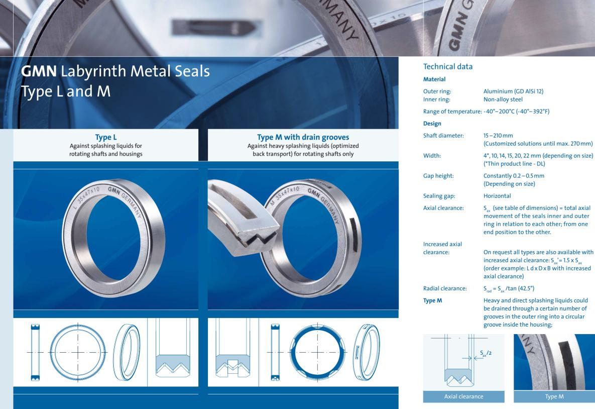
The interlocked labyrinth design keeps inner- and outer ring together as an inseparable unit.
