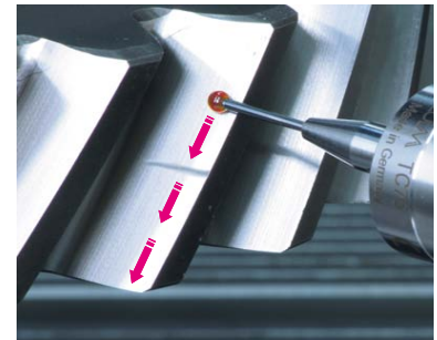
Scanning procedure for checking of workpiece surface
