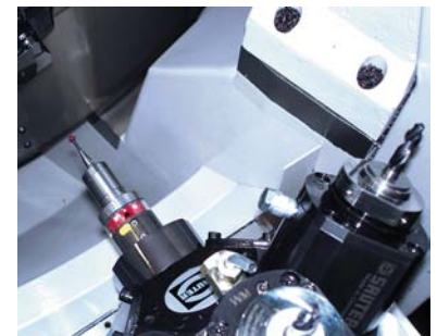
Fast workpiece measurement in rotary transfer machine
